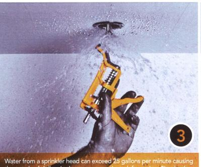
Water from a sprinkler head can exceed 25 gallons per minute causing thousands of dollars in damage every minute left running. Simply place the jaws in the opened sprinkler head with one hand and squeeze the handle once or twice and the water will stop immediately.
